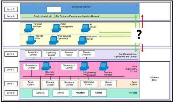
Which product must be positioned where the "?" is placed to connect these different network levels?
